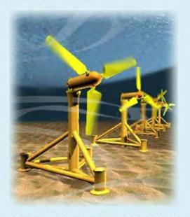
Horizontal Axis Turbine (DEEP-Gen) Source: Tidal Generation
