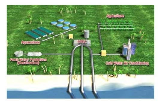
Figure 2-4. Potential co-products of an onshore OTEC electrical energy development. Source: Ocean Engineering & Energy Systems (OCEES), <u>http://www.ocees.com/mainpages/Coproducts.html</u>
