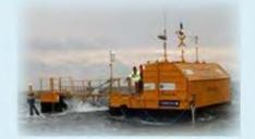
Oscillating Water Column (OEBuoy) Source: Ocean Energy
