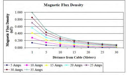
Figure D-2. Calculated magnetic field (A/m) and magnetic flux density ( $\mu$ T) near the WEC submarine power cable.
