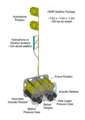
Figure 3-11. Diagram of High Frequency Acoustic Recording Package (a type of passive acoustic monitoring system or PAM) designed and built by the Whale Acoustics Lab at Scripps Institute of Oceanography. Source: NOAA, http://www.pifsc.noaa.gov/psd/mmrp/ cetaceans.php
