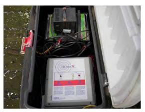
Figure 3-10. Electronic acoustic harassment devices that are used to deter animals (e.g., Pacific harbor seals, California seal lions) from damaging property might also be useful for safely excluding marine mammals, fish, and marine turtles from an ocean energy installation. Source: NOAA
