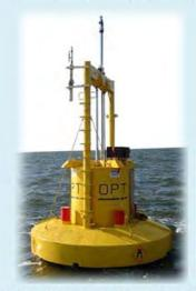
Point Absorber (PowerBuoy) Source: Ocean Power Technologies
